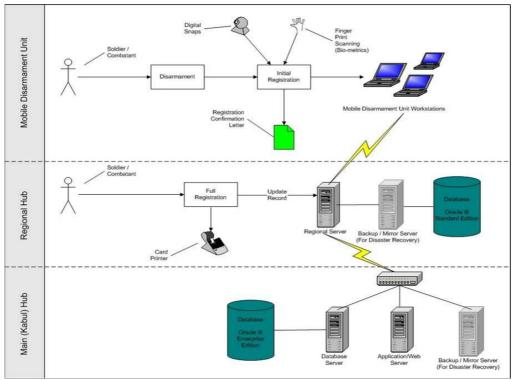
The various devices that were integrated and were part of the solution are Digital Camera, Fingerprint Scanner, 2D Barcode Reader, Card Printer, and Barcode Label Printers.
